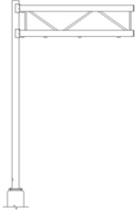
Trussed-Arm Cantilever Structure
