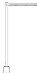
Single-Arm Cantilever Structure
